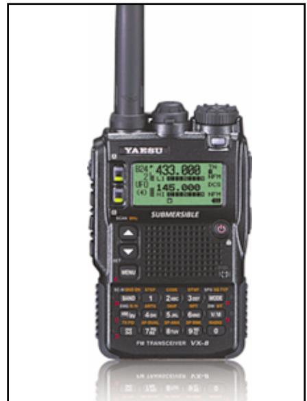
Yaesu has the only quad-band HTs on the market today, the VX-7R and the VX-8DR (pictured). Both cover 6 and 2 meters, plus 222 and 440 MHz. The VX-8DR has a built-in TNC for APRS, and an optional GPS receiver is available.
