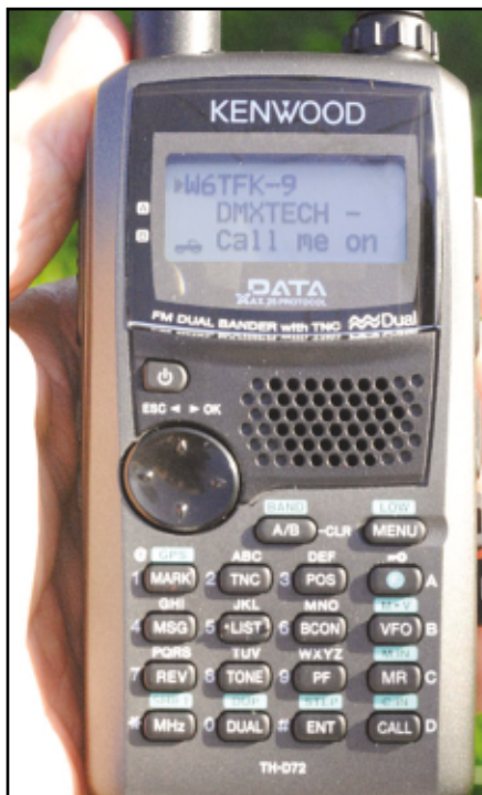
Kenwood's TH-D72 has GPS and APRS capabilities built in. It can also control a TS-2000 HF rig using Kenwood's Sky Command system.
