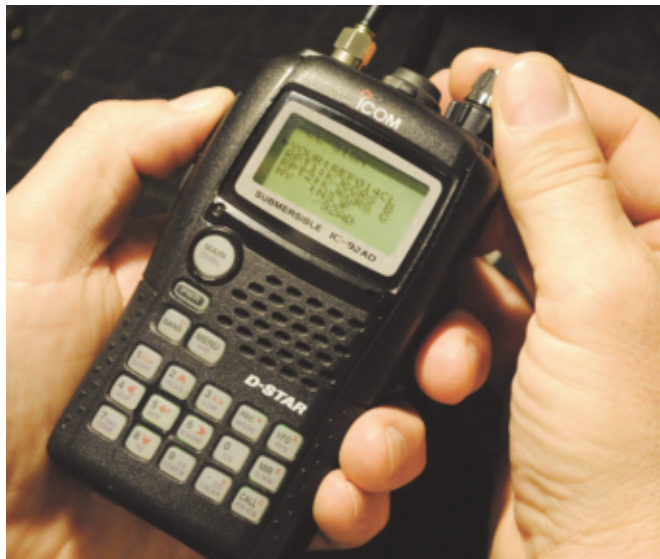
The IC-92AD is ICOM's top-of-the-line dual-band HT, with full-duplex capability for operating FM satellites, and D-STAR capability built in. You can also get an optional GPS microphone.
