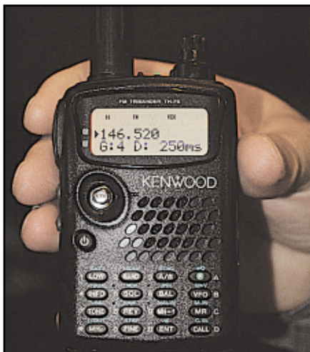
The popular Kenwood TH-F6A covers the 222-MHz band as well as 2 meters and 70 centimeters, with broadband receive (including CW/SSB) from 100 kHz to 1300 MHz.
